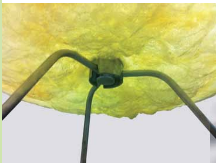
Fig. 1 and 2: Prototype tables made with Glycix, a new biobased material developed by the University of Amsterdam.
